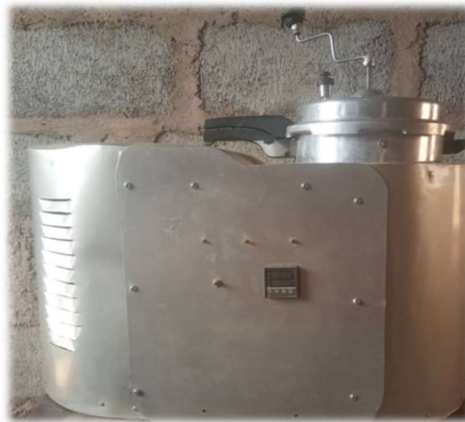
Fig A3. First fabricated model of the Automated Yam cooking and pounding machine with integrated spring doneness tester.
